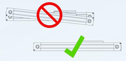
Actual tolerances related to alignment recommendations and mounting vary from actuator series. Profile ball rail systems tend to be quite rigid and alignment is more critical. Guide wheel units often have clearance, which offer some forgiveness in alignment.
